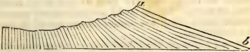
When strata protrude above the surface of the ground, as at *a*, they are said to *crop out*, and the angle at which they incline below the horizon is their *dip*; the *thickness*, of course, is the perpendicular distance between their upper and under surface. Some rocks, particularly slates, are subdivided by numerous vertical joints, dividing the whole mass into cubical or rhomboidal masses, as in the following cut:
